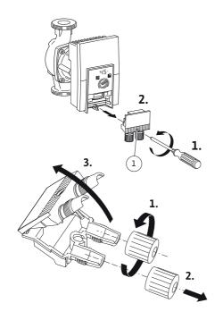
Use a screwdriver to remove wiring box from the pump head.
