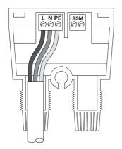
Wiring from IMM into the wiring box. Wire to the Live, Neutral and Earth terminal blocks.
